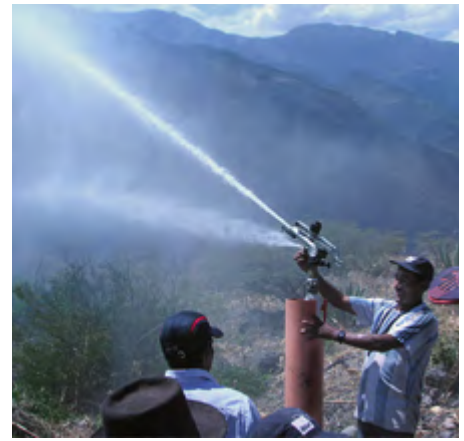
The sprinklers project water in a 40 m radius
